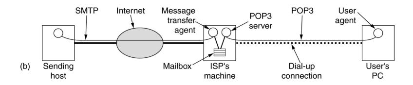
(a) Sending and reading mail when the receiver has a permanent Internet connection and the user agent runs on the same machine as the message transfer agent. (b) Reading e-mail when the receiver has a dial-up connection to an ISP.
