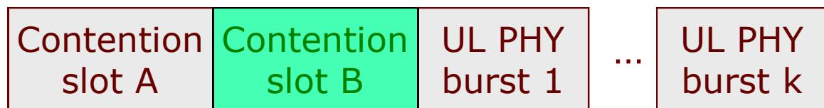
The usage of **bandwidth request messages** in this contention slot (and **response messages** in downlink bursts) offers a mechanism for achieving extremely flexible and dynamical operation of IEEE 802.16 systems.
