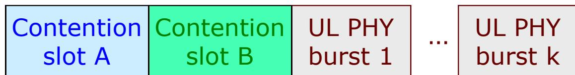
The uplink subframe starts with a contention slot that offers subscriber stations the opportunity for sending **initial ranging messages** to the base station (for timing and power control adjustments).
